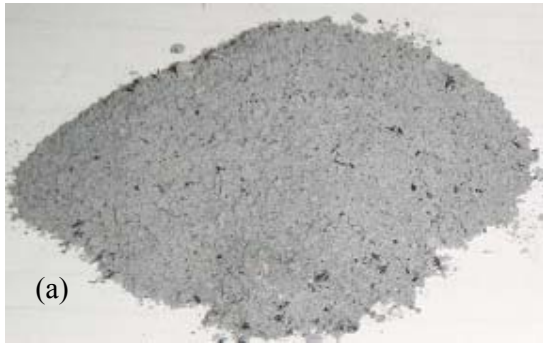
Fig 9: Photograph of grass pellet ash for this study (a), and grass briquette ash from conventional wood stove (b)
